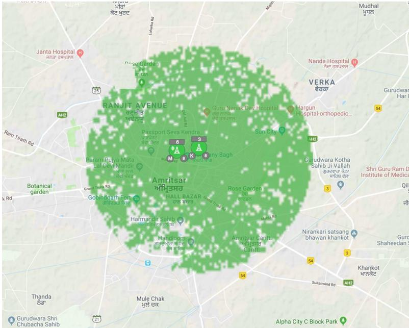
Figure 5: LoRaWAN™ Gateway Site 1 (micro-cell gateway)
